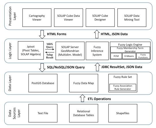
Figure 2. Multilayer framework architecture of FSOLAP.
