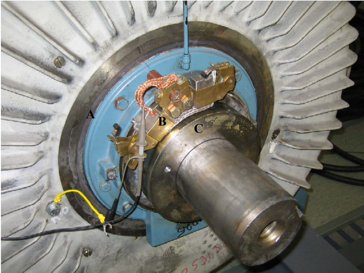
Fig. 5.1. End shield of the motor used in the experiments: insulation ring (A), copper brush (B), and slip ring (C).
