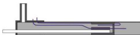
Fig. 11 Schematic of the microseparator used in industrial measurements; contaminated air inlet from the right hand side
