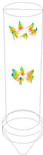
Fig. 10 Schematic of the industrial tower with dispersed phase injection regions, Wawrzyniak et al. (2012a, 2012b)
