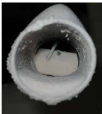
Fig. 13 Particles build-up on the outer tube of the microseparator
