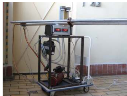
Fig. 12 Experimental set up for microseparator measurements in the industrial tower
