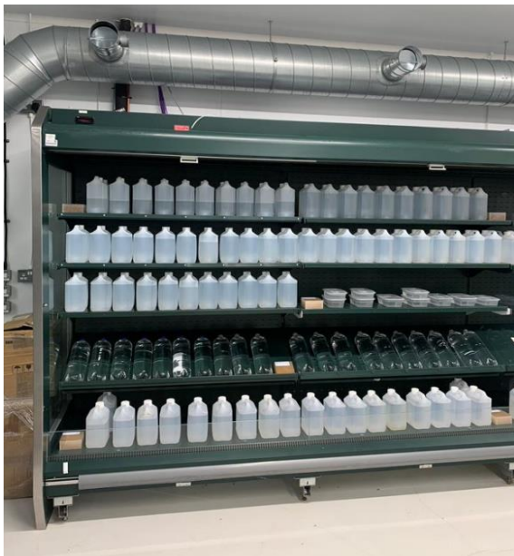
Figure 3: High temperature (HT) Monza display case used at Risholme Refrigeration Research Centre.
