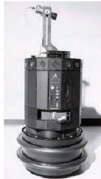
Fig. 6. The Nomad 200 is a mobile robot equipped with a ring of 16 sonar sensors.
