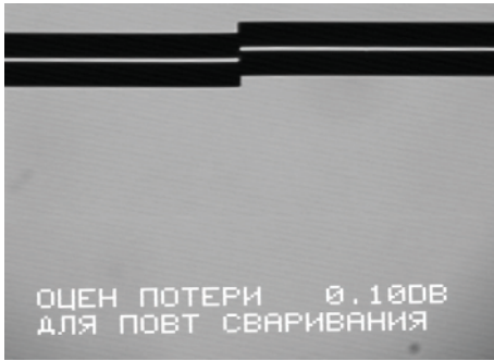
FIGURE 12: Screenshot of the Ericsson FSU-975 display with offset fusion splice.
