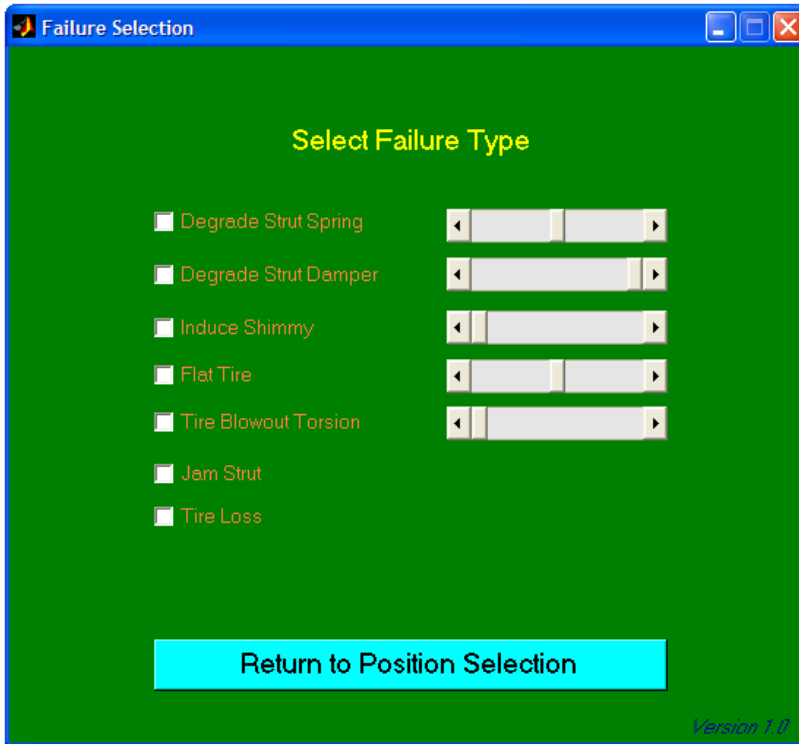
Figure 28. Depiction of possible nose failures.
