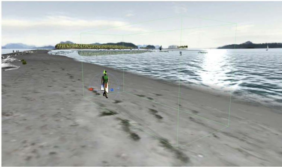
FIGURE 12 | Person model equipped with sound collider. Green box around the person model represents a sound collider. When the user character enters the collider, a greeting sound is triggered, giving the user the sense of being greeted by another park visitor.
