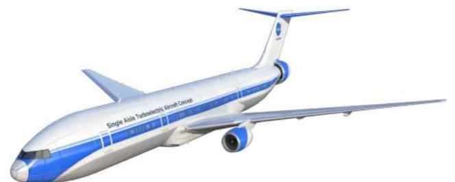
Fig. 1 NASA’s STARC-ABL aircraft concept, incorporating a hybrid-electric propulsion system and aft-mounted BLI propulsor [4].
