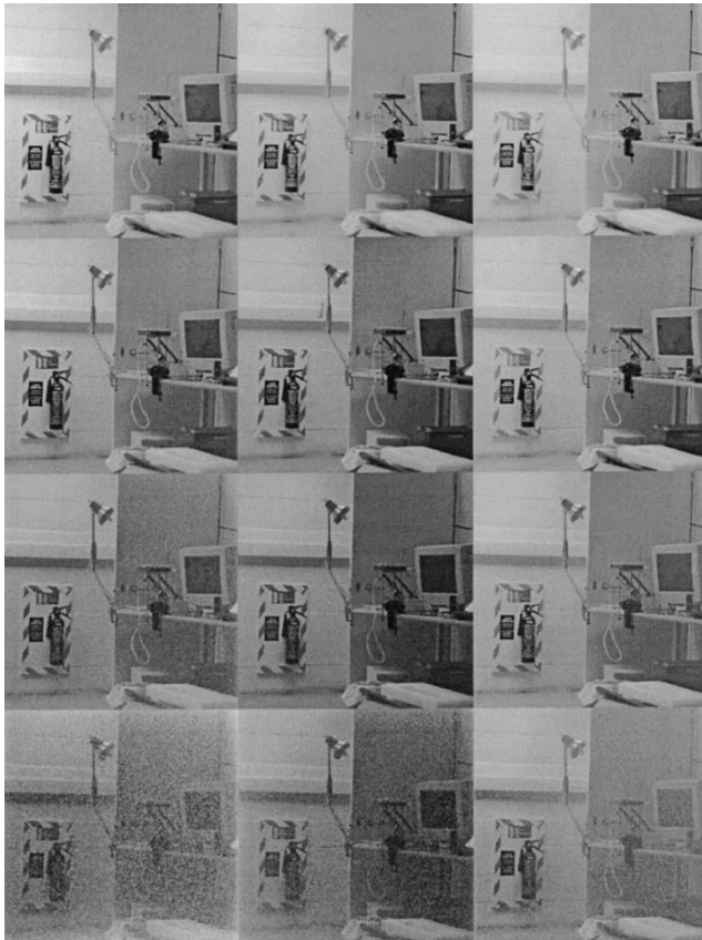
Fig. 4. A scene, using single, double, and triple variation correction (left to right), imaged with apertures of 1.8, 4, 8, and 16 f-stops (top to bottom).
