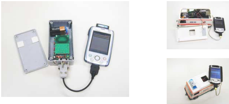
Fig. 5. RFID reader with PDA device and a model emergency car with sensor equipment.
