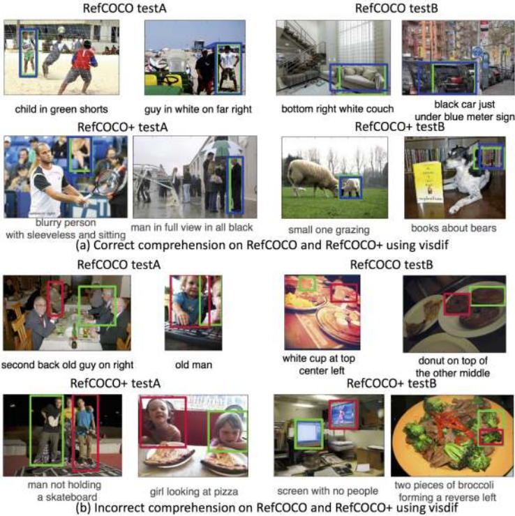
Fig. 3. Some examples showing comprehension results of visdif+MMI based on detection. The blue and red bounding boxes are correct and incorrect comprehension respectively, while the green boxes indicate the ground-truth regions. (Color figure online)
