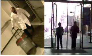
Fig. 2. The left panel shows an example of a double count at the loading dock entrance of the building; the right panel shows an example of a missed count at the front door.
