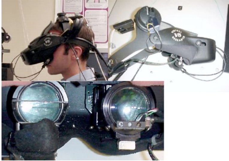
Fig. 9. The head mounted display worn by human subjects has eye tracking capability so that gaze can be tracked in virtual environments. The display has a 55^\circ diagonal field of view.)
