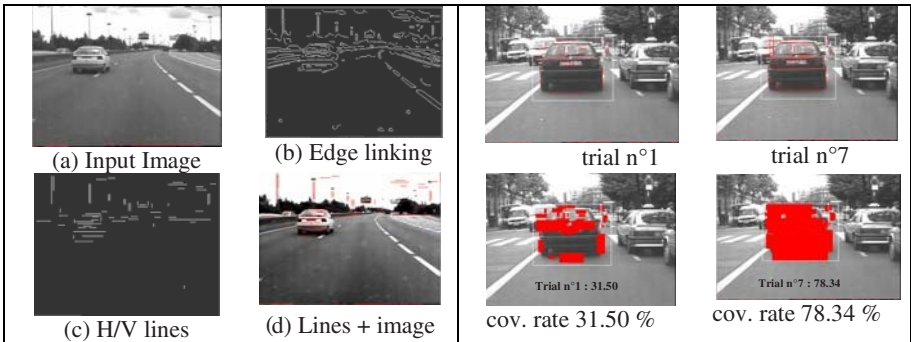
Fig. 3. H/V line Extraction (left) and IPC Output evaluation (right)
