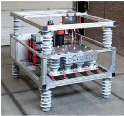
Fig. 4. Prototype of VARC dc CB.
