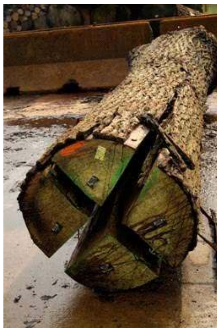
Fig. 1.2 A logged tree which has cracked due to the release of growth stresses. Picture taken from [43].
