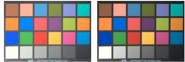
Figure 11: Our model can be used to match the color appearance on different media. Starting from a radiometrically calibrated XYZ float image [Kim and Kautz 2008], the left image printed on paper will appear very similar to the right image when displayed on an LCD (assuming calibrated devices in dim viewing conditions).
