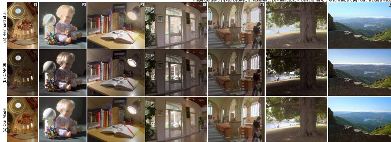
Figure 13: Absolute HDR radiance maps are tone-mapped using Reinhard et al.’s tone-mapping algorithm [2002], the iCAM06 image appearance model [Kuang et al. 2007], and our color appearance model. The target display is assumed to be sRGB with a peak luminance level of 250 \text{ cd/m}^2 and a gamma of 2.2 (dim viewing conditions, adapting luminance is assumed to be 10% of peak luminance). For Reinhard et al.’s and our method, we simulate chromatic adaptation as outlined in Section 5.1; iCAM06 uses its own spatially-varying model.
