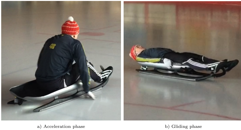
Figure 4: Procedure of the ice house experiments. The athlete accelerates the sled similar to a luge starting phase. Friction is measured during the gliding phase.
