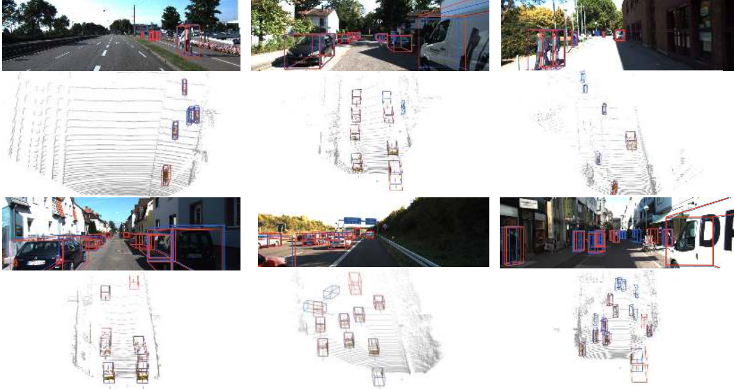
Figure 4. We visualize the detection results on KITTI with 2D and 3D images. The red boxes are the groundtruth boxes and the blue boxes are the prediction results. Some of the false positive detection results are because of missing annotation.
