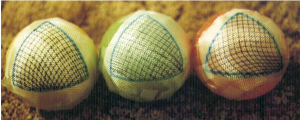
Figure 8: Fitting results with an actual sheet of woven cloth fiberglass
