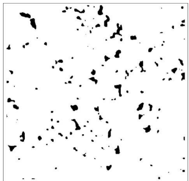
Fig. 2 Binary image of tight sandstone used for modeling (100 × 100 pixels, white is solid, and black is void)
