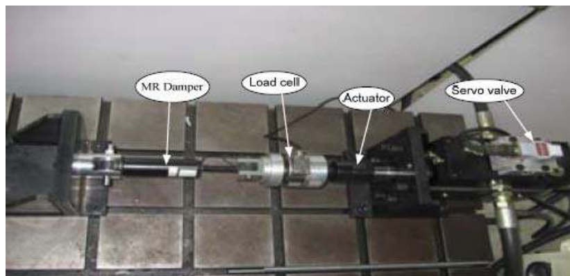
Fig. 4. RD-1005-3 damper in the test rig
