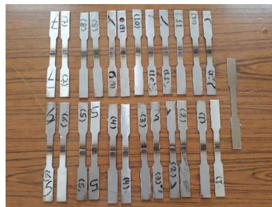
Fig. 5. Rectangular cross-section tensile test specimen according to ASTM E8-M. [1°] All dimensions are in millimeters.
