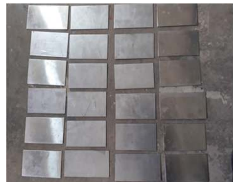
Fig 1. Weld specimen's preparation.
