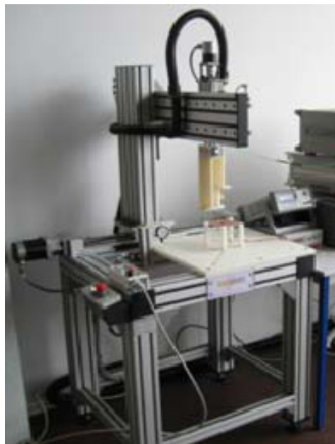
Figure 10. Photograph of the IRSEEM test bench used for the magnetic NF measurement
