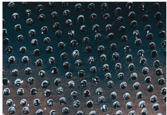
Fig. 1 LST regular micro-surface structure in the form of circular micro-dimples each is having a diameter of the order 100 \mu\text{m} and a depth of the order of 1–10 \mu\text{m} .
