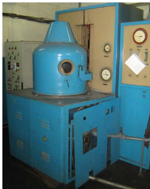
Fig. 1. A general view of the NPI 6.6/6 furnace for ion-plasma nitriding
