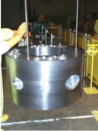
Fig. 34. Views of the permanent beryllium reflector.
