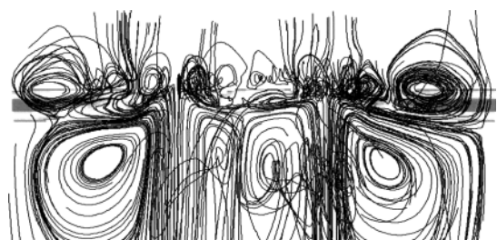
Fig. 16. Path lines in flow field near the zone of slag layer.
