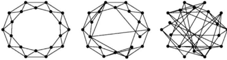
Figure 3.1: The initial configuration for the Watts and Strogatz model with n = 20 and k = 4 (left); the resulting network for some 0 < \beta < 1 (middle); and the resulting network for \beta \approx 1 (right). Diagram reproduced from [22].
