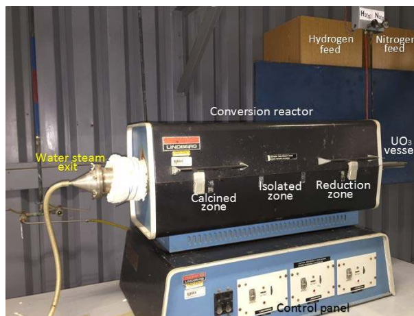
Figure 4. UO 2 conversion reactor.
