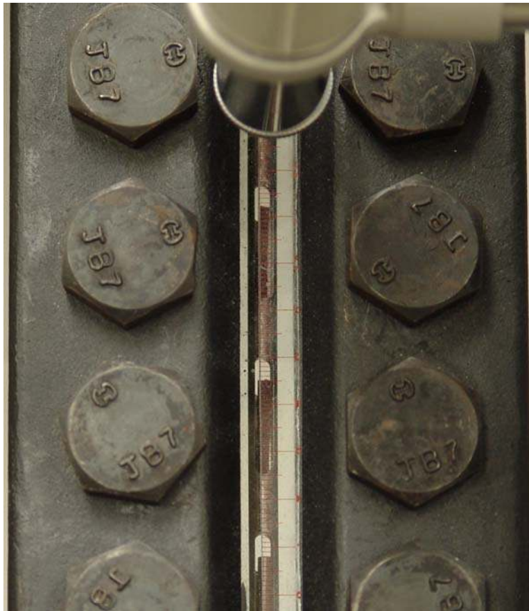
Figure 4.6. Photograph of clear measurement standard overlaying the clear glass wall of the pressure vessel. At the top of the figure the bottom of the microscope can be seen; in the center, the sample holder containing coal samples.
