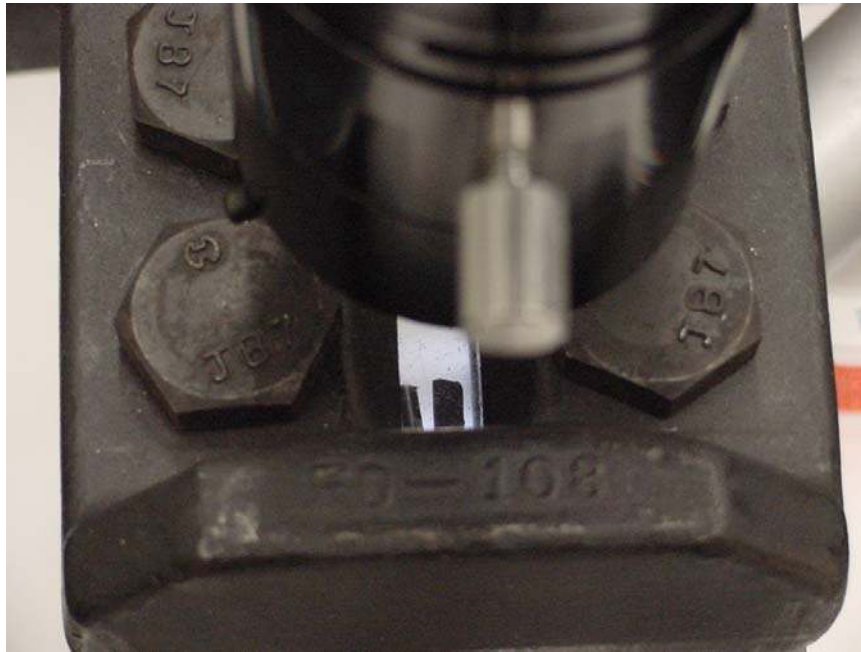
Figure 4.2. Close up view of the pressure cell and video camera lens. Inside the pressure cell can be seen the ends of a piece of 1/8-inch stainless steel tubing (left) and a piece of coal (right).
