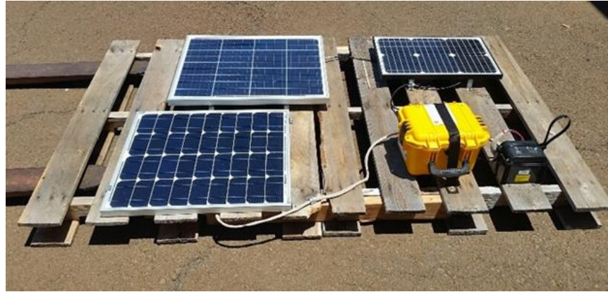
Figure 2. The assembled test system in the field. The polycrystalline solar panel is positioned at the top right with the monocrystalline panel below it. The yellow waterproof case is present as well. The external battery and the third panel to charge the battery are each in the bottom right and top right of the photo, respectively. [4], [9]
