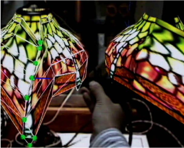
Figure 12. Deforming the model by translating selected vertices.
