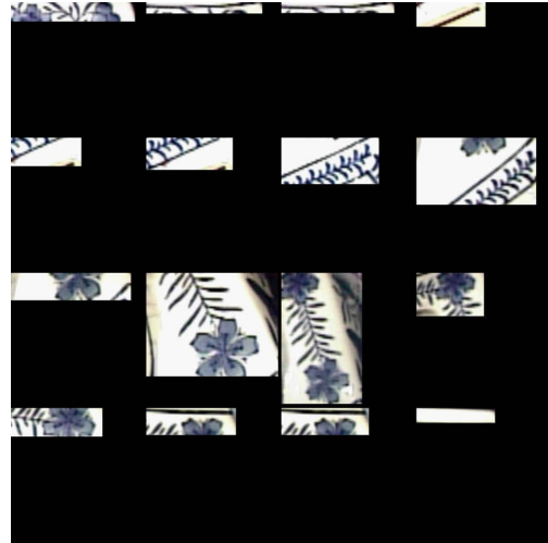
Figure 9. Stored texture array. These are the textures used to render the model interactively. Each rectangular texture corresponds to the bounding box of a triangle.
