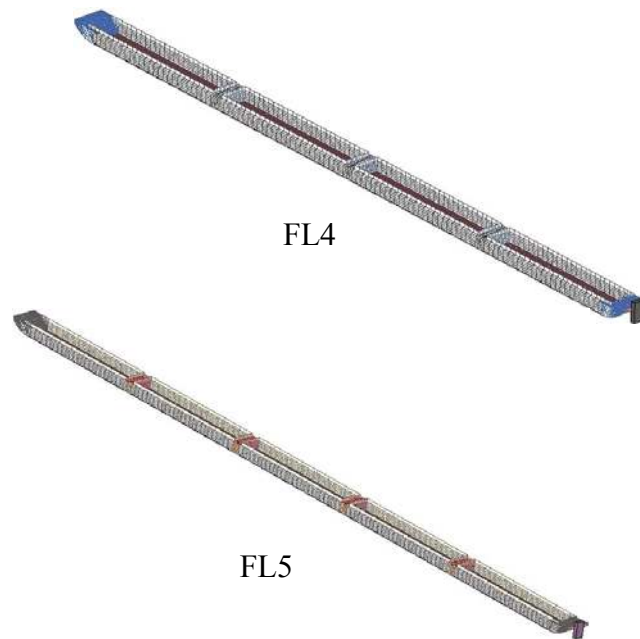
Figure 6.13 FE models for FL4s and FL5s
