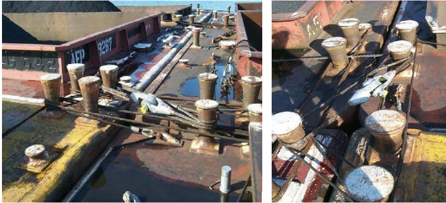
Figure 6.4 Wire ropes connecting barges in a multi-barge flotilla
