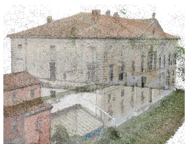
Figure 5. The Achieved point cloud obtained using UA Vand terrestrial data in the external part of Palazzo Sarmatoris.
