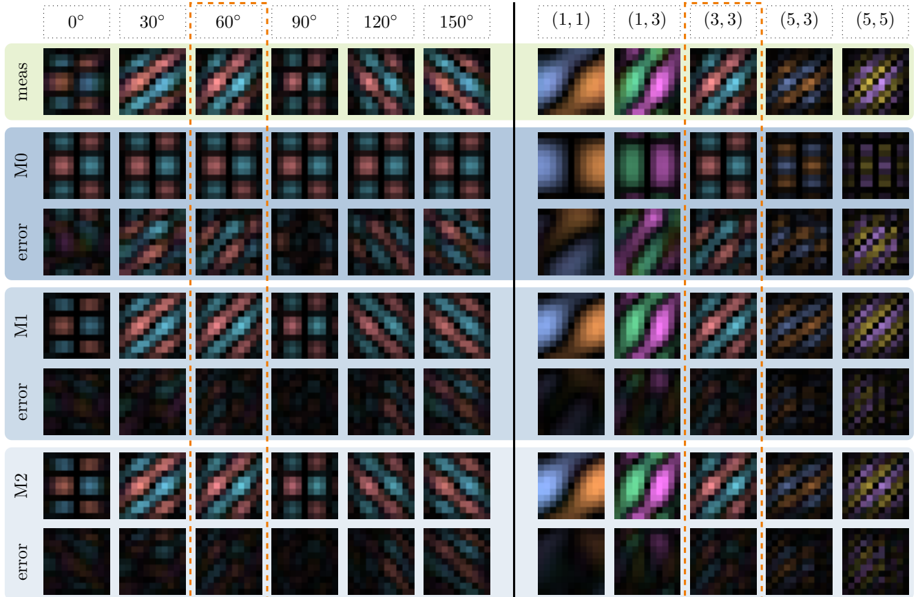
Figure 5: Comparison of the modeled MPI system matrices for models M0 to M2 with the measured system matrix for the x -channel. The left part of the figure shows a comparison for a fixed frequency component ( m_x = 3, m_y = 3 ) and various angles in 30^\circ steps. The right part of the figure shows the data for a fixed angle of 60^\circ and several frequency components at mixing orders (m_x, m_y) \in \{(1, 1), (1, 3), (3, 3), (5, 3), (5, 5)\} . The orange dashed box indicates the data that is present in both parts of the plot. In addition to the matrix patterns itself, the complex-valued difference D_{k,\theta} = S_{k,\theta}^{\text{model}} - S_{k,\theta}^{\text{calib}} is shown. All data uses the complex colormap shown in Fig. 1 whereas the same windowing is used for each frequency index k .
