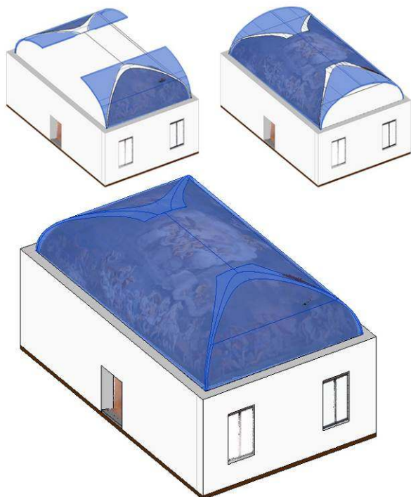
Figure 3: Vault construction by successive subtraction of solids.
