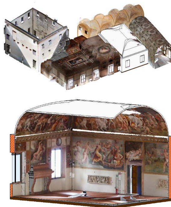
Figure 1: (top) the 3D model of Sala di Troia with all the point clouds of Apartment di Troia, (bottom) point cloud integrated in Revit environment.
