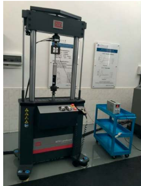
FIGURE 2: (a) Schematic of the experimental setup. 1, data acquisition system; 2, PC; 3, the force sensor; 4, MTS370; 5, rod; 6, aluminum shell; 7, cylinder of MR damper; 8, MTS370 actuator; 9, the inner displacement sensor; 10, rod (connected to anode of current source); 11, copper needle in rod (connected to cathode of current source); 12, current source (Qiujiing QJ3005T). (b) Test rig.
