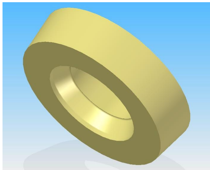
Figure 2. Model of Draw Die (seizing plate)
