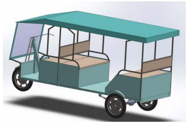
Fig. 1 SolidWorks ® model structure of the proposed three-wheeled vehicle
