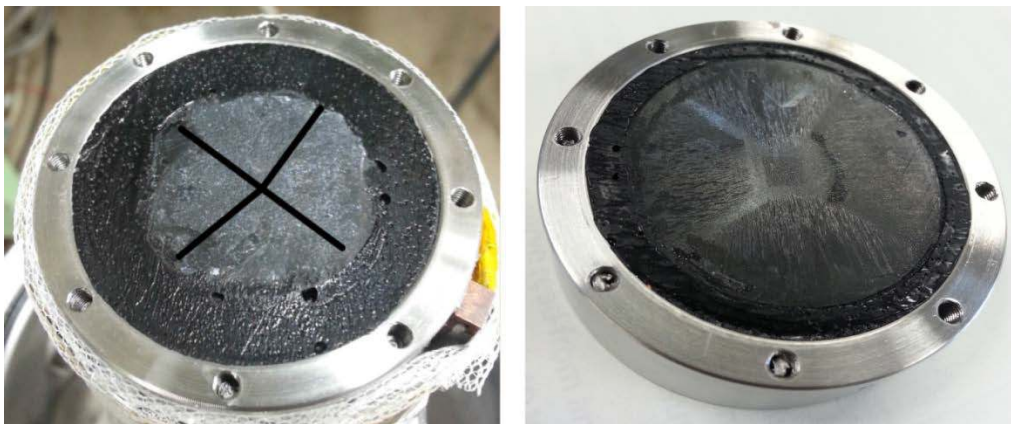
Figure 1. YBCO (left) and GdBCO (right) bulk superconductor samples. The growth sector boundaries (GSBs) are shown in each sample.
