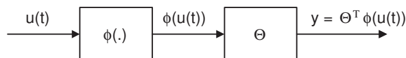
Figure 8.1. The dynamic model is linear with respect to the dynamic parameters and can be expressed as a linear regression model.
