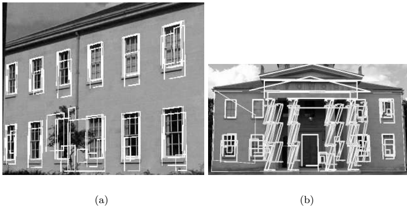
Figure 9: Collection of shapes whose likelihood ratio of being a window to not being a window is high. The zig-zag shapes correspond to columns.
