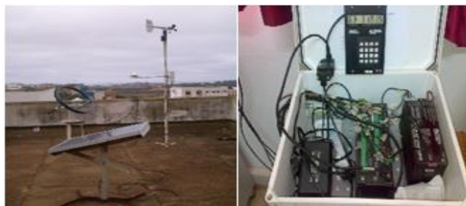
Figure 2. Meteorological Station Campbell Data Logger CRX10X
