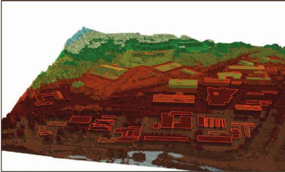
Figure 7. TIN created from photogrammetry and LiDAR.
