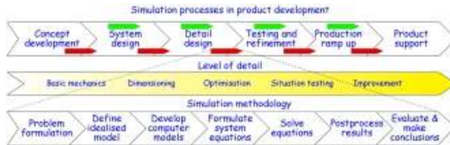
Fig. 3. Simulation methodology in different phases of the development process.
