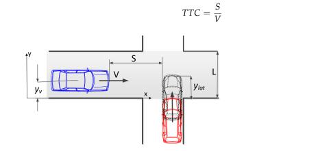
Figure 1. Scheme of a road situation.
