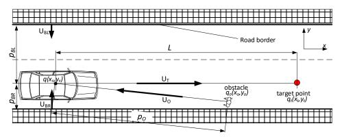
Figure 2. Scheme of interactions in the potential field.
