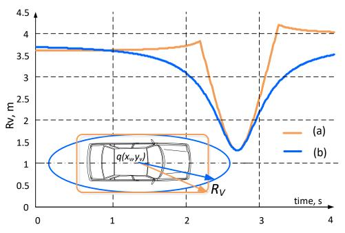
**Figure 6.**  $R_V$  parameter change depending on the shape of the safety zone around the vehicle: (a) rectangle, (b) ellipse.
