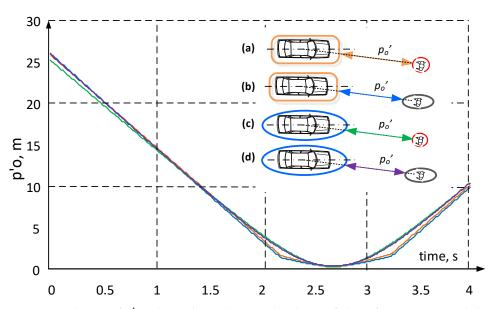
**Figure 7.** Change of p'o values, depending on the shape of the safety zone around the vehicle and the obstacle: (a) vehicle—rectangle, obstacle—circle; (b) vehicle—rectangle, obstacle—ellipse; (c) vehicle—ellipse, obstacle—circle; (d) vehicle—ellipse, obstacle—ellipse.
