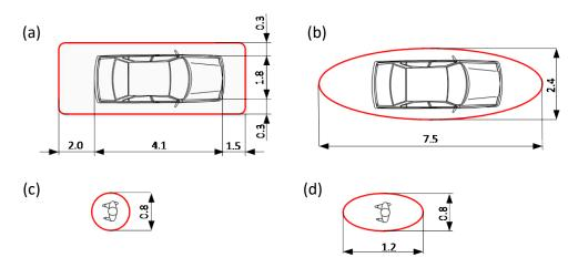
**Figure 5.** Size of the safety zone dimensions used in the simulation; (**a**) vehicle rectangular, (**b**) vehicle elliptical, (**c**) pedestrian circular, (**d**) pedestrian elliptical.
