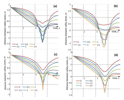
**Figure 8.** Distance in *y*-axis direction between safety zones for different lateral speeds (km/h) of the obstacle: (**a**) vehicle—rectangle, obstacle—circle; (**b**) vehicle—rectangle, obstacle—ellipse; (**c**) vehicle—ellipse, obstacle—circle; (**d**) vehicle—ellipse, obstacle—ellipse.
