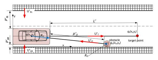
Figure 4. Introduction of vehicle and obstacle safety zones to the situation scheme.
