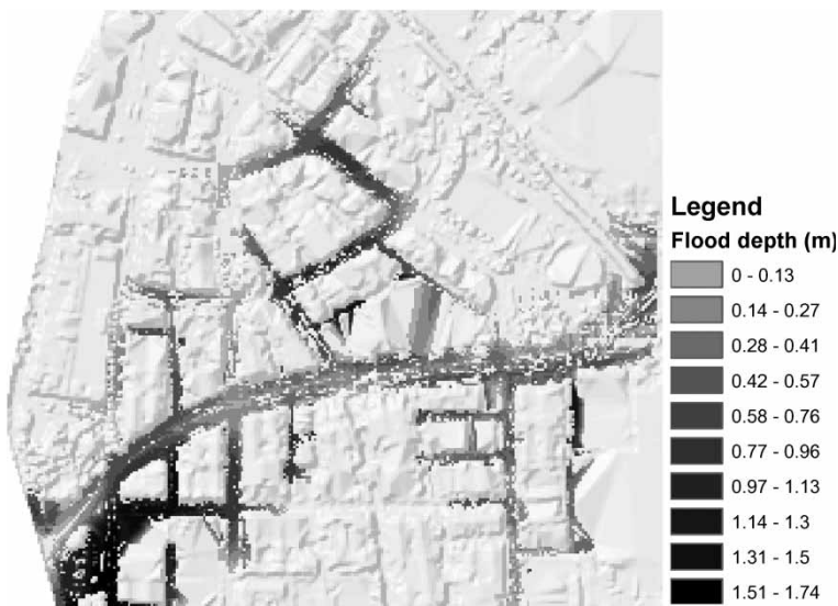
Figure 20 | Maximum flood depth for the coarse grid ( 10 \times 10 m) model using the method based on adjusted conveyance and storage characteristics.
