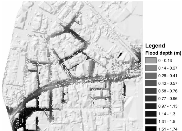
Figure 21 | Maximum flood depth for the coarse grid ( 12 \times 12 m) model using the method based on adjusted conveyance and storage characteristics.
