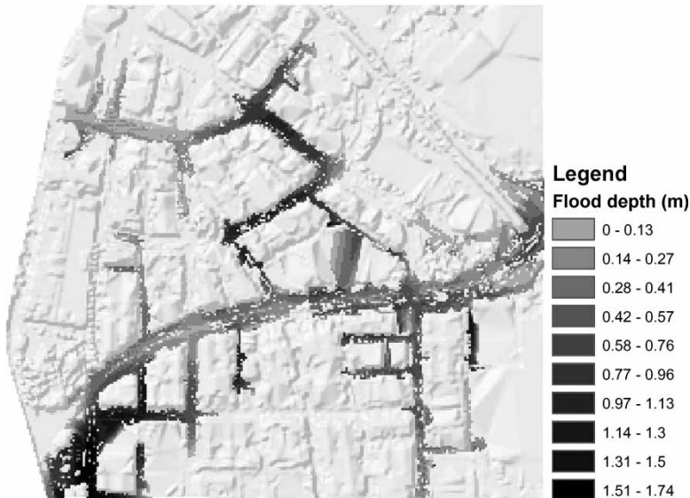
Figure 15 | Maximum flood depth for the fine grid ( 2 \times 2 m) model using the straightforward 2D modelling approach.
