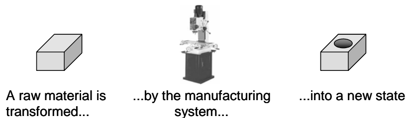
Figure 13: The manufacturing system is able to perform changes of a material
